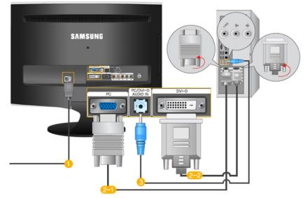
Connect the power cord for your monitor to the POWER port on the back of the monitor.
